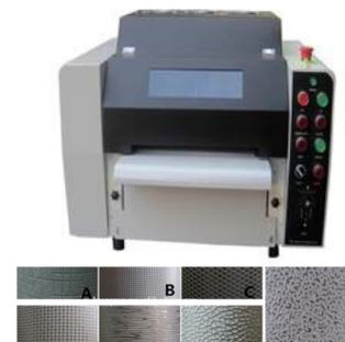
DPL-UV200-LFD also can be connected into your existing printing press as the final surface finishing process.
